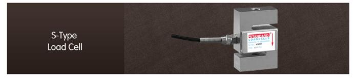
These are staingage based loadcells designed for both tension and compression loading, they are made from high tool steel alloy with Electroless nickle platting for protecting loadcells from jerk loads & corossion. These loadcells are IP67 protected. They are used for electronic scale modified from mechanical scale, Hopper scales, force measuring systems, industrial weighing and control system.
